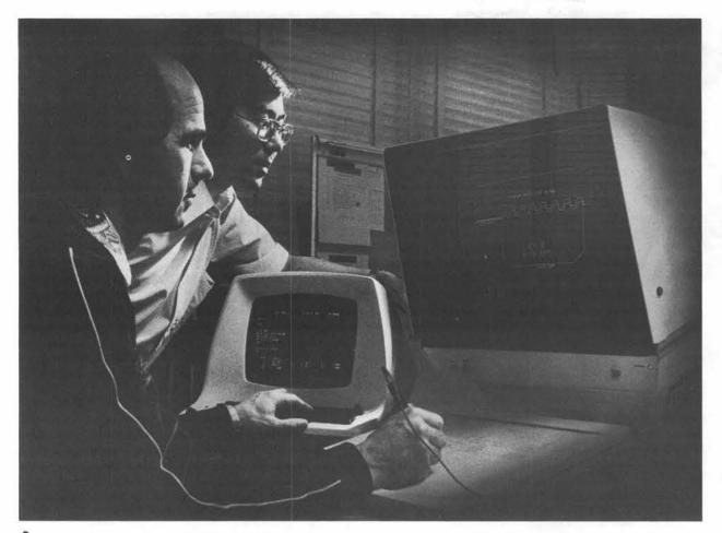
DESIGNING BY COMPUTER — Vern Byfield (8274) uses an electronic pen and a keyboard to modify a design on the CRT to engineer Howard Hirano's (8441) satisfaction. The CADDS system offers a wide range of graphic options to the designer.
